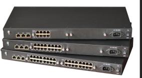
TPG Analog VoIP Gateways are cutting-edge products that connect legacy telephones, and PBX systems with IP telephony networks and IP-based PBX systems. Featuring rich functionalities and easy configuration, TPG is ideal for small medium & large enterprises that wish to integrate a traditional phone system into IP-based system. TPG helps them to preserve previous investment on legacy telephone system and reduce communication costs significantly with the true benefits of VoIP.
